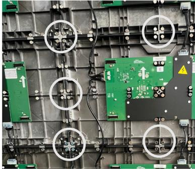
8. Repeat **Step 1~7** for the remaining Cabinets, ensuring that the Mounting Brackets sit securely on the Wall Mount Brackets, and that the Cabinets are properly secured together.
