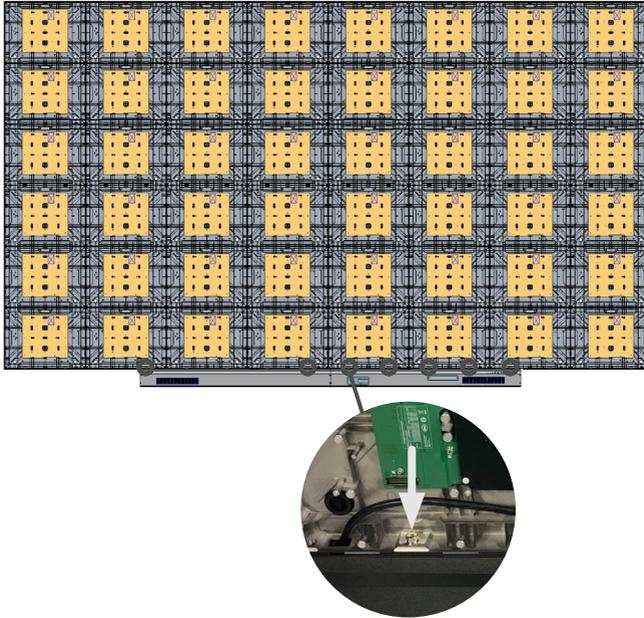
7. Connect the Power and Network Cables of the Cabinets from the System Control Box to each Cabinet. Start from the bottom and move to the top (see Appendix B for example system wiring diagrams, including wire colors and connection points).
